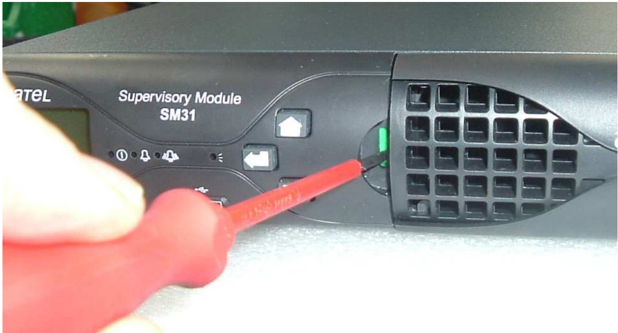
Fig 4. For removal, unlock SM3x by lifting green locking tab.
